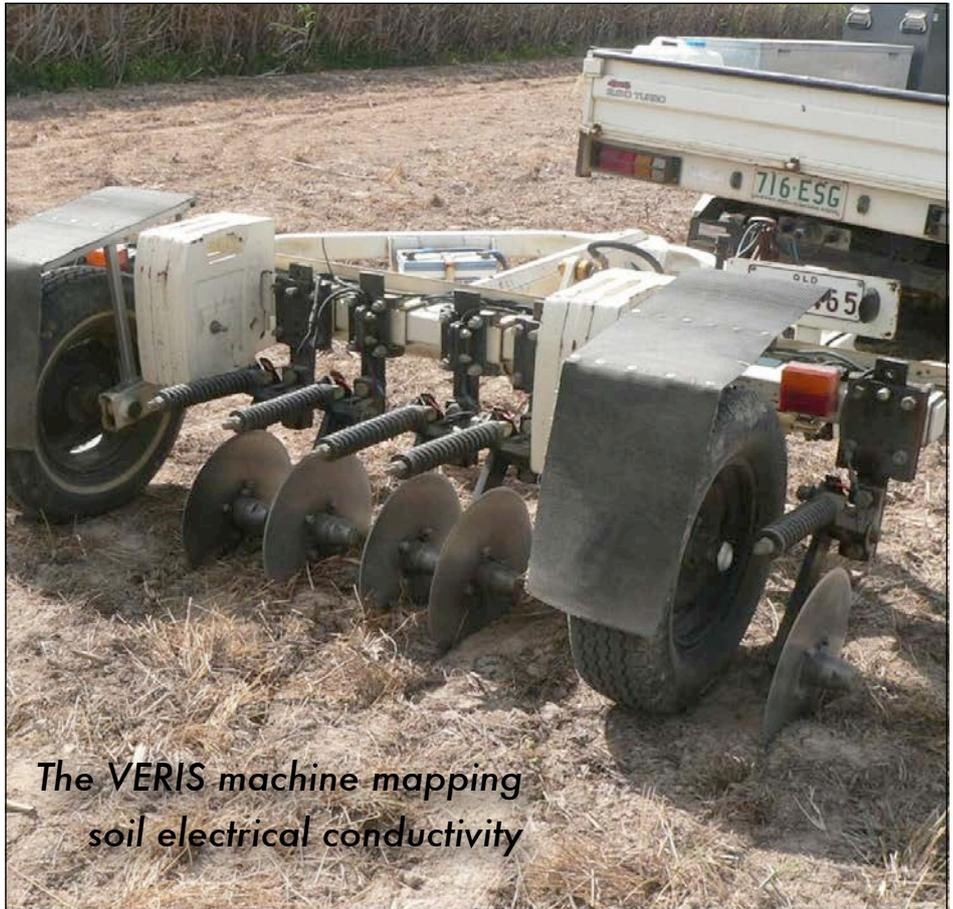
*The VERIS machine mapping soil electrical conductivity*
